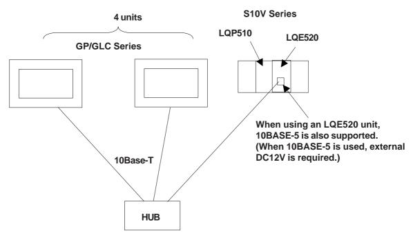
\* Communication is fixed as TCP format.Maximum number of GP units is 4, based on PLC specifications.
