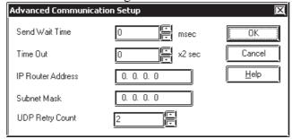
\* Since communcation settings are designated in the PLC specifications as TCP, setting the UDP Retry Time is not required.
